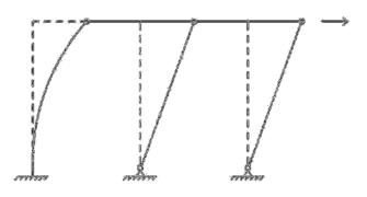
Figure 3.5: A lean-on system of columns.
