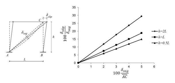
**Figure 3.22:** An example of how the sag of a diagonal member would require that a movement  $(\delta_{slip})$  at the top of the frame take place in order for the diagonal to be activated (i.e. straigthened out).
