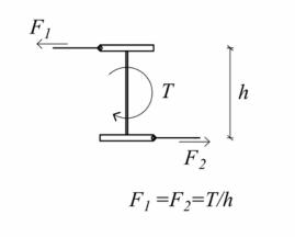
Figure 3.6: Torsional bracing of an I-girder as achieved by means of two translational bracings, i.e. by the force couples  $F_1$  and  $F_2$ . It is assumed that the bracings can take both tension and compression.
