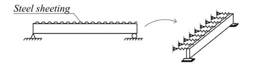
Figure 3.3: Continuous bracing of a beam by decking (with use of a corrugated steel sheet).
