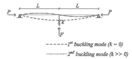
Figure 3.7: A braced strut.
