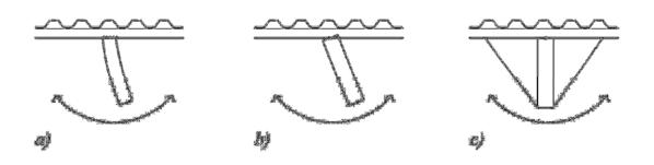
**Figure 2.9:** A primary beam in a roof structure rotating around its longitudinal axis due to negative bending: a) torsional rigidity being provided by the purlins and the roof cladding, b) the joint between the primary beam and the purlin being a pinned one, and c) torsional bracing of the cross section being provided by means of tension ties connected to the bottom side of the member.
