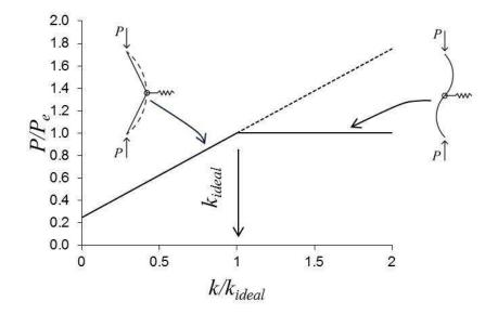
Figure 3.9: The elastic buckling capacity of a braced strut shown as a function of the brace striffness,  $k_{ideal}$  is the ideal bracing stiffness, and  $P_e$  is the the Euler buckling load when buckling between successive restraints occurs.
