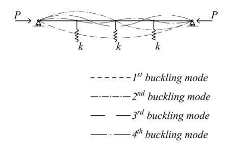
Figure 3.11: Buckling modes of a strut that is being braced at three points.
