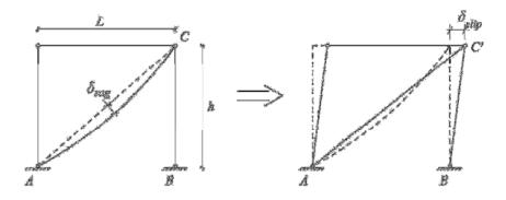
Figure 3.20: An illustration of how a sagging diagonal needs to be straightened our before it can resist a lateral load.
