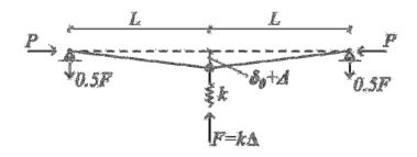
**Figure 3.12:** A rigid link model involving an initial imperfection ( $\delta_0$ ).
