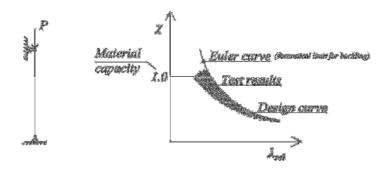
**Figure 3.1:** A schematic diagram of a typical design curve for the design of columns:  $\lambda_{rel} = \sqrt{N_p/N_{cr}}$  and  $P_u = \chi N_p$ .  $N_p$  being the plastic capacity of the column,  $N_{cr}$  the Euler buckling load, and  $P_u$  the "capacity" of the column.
